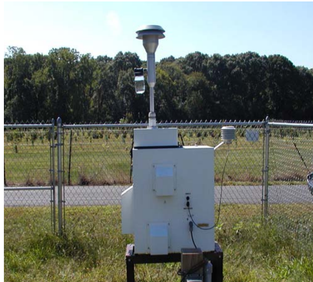
Ambient air monitoring fine particle sampler located at the New Brunswick Site in Middlesex County.
